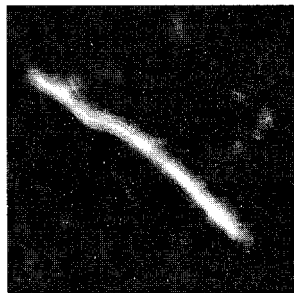
Fig. 1. AFM topographic image (200nmX200nm) of an insulated molecular wire formed by the \alpha -CD nanotube and PANI. The length is almost equal to the average contour length 300nm of PANI and the height is close to the outside diameter of \alpha -CD.
